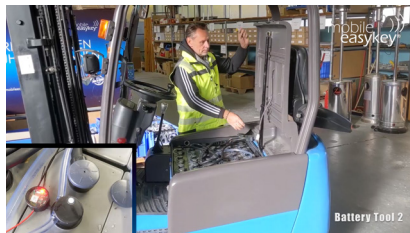
Warning by red LED on the electrolyte sensor
